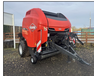
NEW New Kuhn VB 3260 OPTICUT, integral rotor with Harbox tines, 14 selectable knives, drop floor, ISOBUS control. £POA
