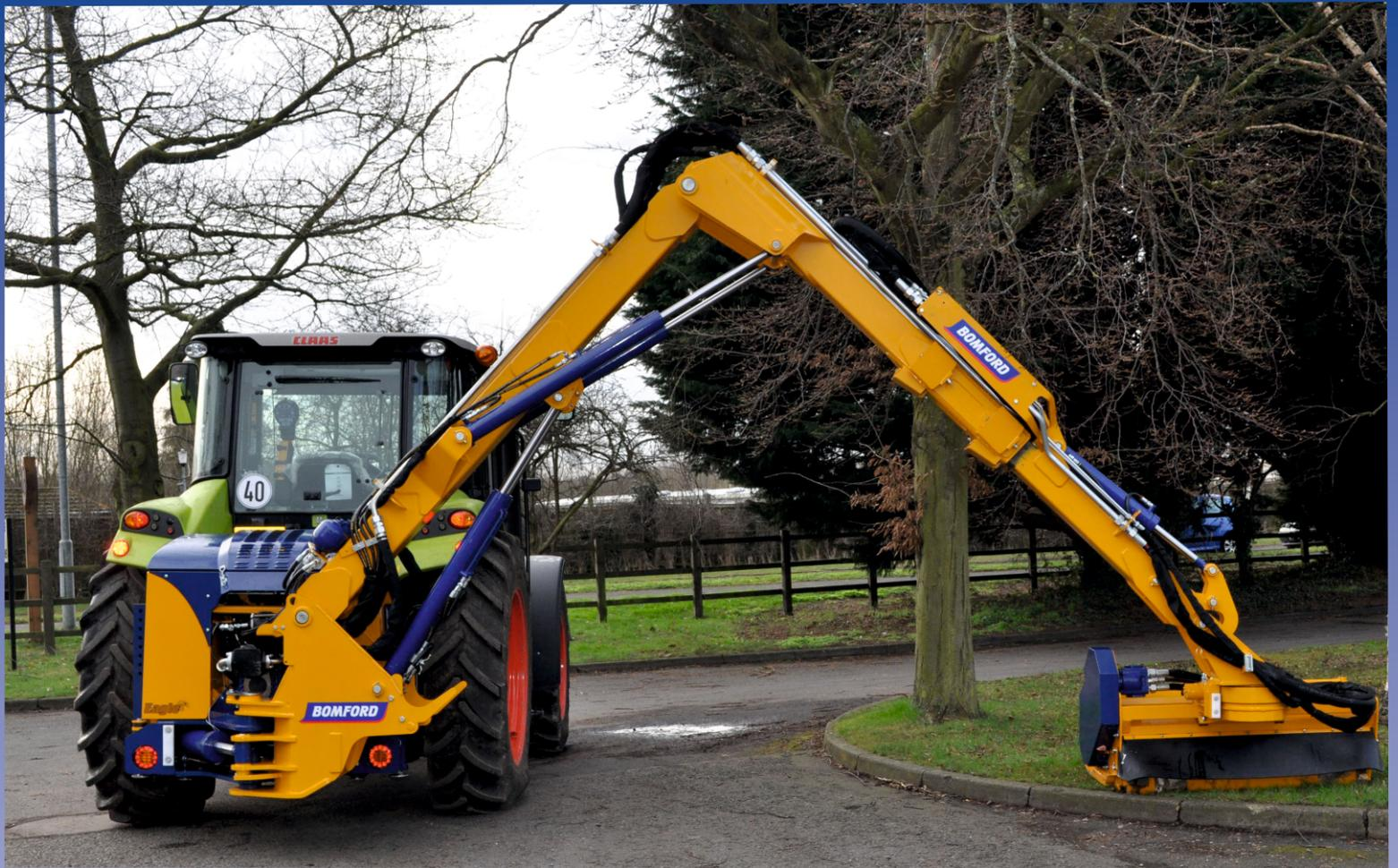
The Eagle flail mower is a 137 litre per min, 8.0m reach, non-parallel geometry, twin sided cutting straight arm machines with a telescopic outer arm and a hydraulic turntable for the attached implement. These durable professional contractor machines have a separate mainframe and oil tank and also a kingpost which allow's the arm set to be slewed through 180 degrees for twin cutting, left hand and right hand.
